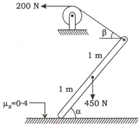
A rod of length 2 m and weight 450 N rests on ground at one end. The other end is supported by a cord through which a force of 200 N is applied. What is the minimum angle  $\alpha$  for which equilibrium is possible? The coefficient of static friction between the rod and the floor is 0.4 :
