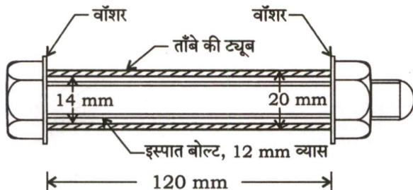
Two thick washers are placed on the two ends of a copper tube and a steel bolt of pitch 1.8 mm is made to pass through these washers as shown in the figure below. The nut is tightened first with hand so that there are no stresses in the tube. Now, the nut is further tightened with the spanner through one-fourth of a turn. Calculate the axial stresses developed in the tube and the bolt. Young's modulus values for steel and copper are 200 GPa and 105 GPa, respectively :
