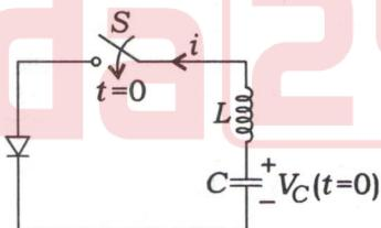
A diode circuit with an  $L-C$  load is shown in the figure, with the capacitor having an initial voltage  $V_C(t=0) = 120$  V, capacitance  $C = 12 \mu\text{F}$  and inductance  $L = 48 \mu\text{H}$ . If switch  $S$  is closed at  $t = 0$  s, then find the following :
