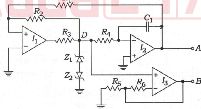
Suggest to replace suitable resistances so that the output voltages at A and B are having swing of  $\pm 6 \text{ V}$  and the output frequency is fixed to 500 Hz.
