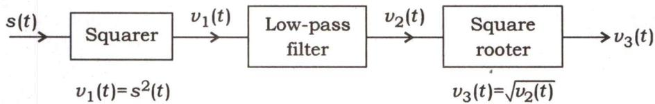
Assume that  $|k_a m(t)| < 1$  for all  $t$ , the message signal  $m(t)$  is limited to the interval  $-\omega \leq f \leq \omega$ , and the carrier frequency  $f_c > 2\omega$ .
