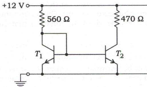
In the circuit diagram given here,  $T_1$  and  $T_2$  are transistors with matched characteristics. The transistor parameters in active region are  $\beta = 200$  and  $V_{BE} = 688 \text{ mV}$ . Find  $V_{CE}$  of transistor  $T_2$  :
