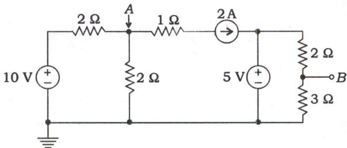
Find the voltage on points A and B of the given circuit :
