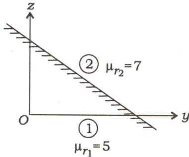
In the figure given below, region 1 is the side of the plane  $y+z=1$  containing the origin and in this region,  $\mu_{r_1} = 5$ . In region 2,  $\mu_{r_2} = 7$ . It is given that  $\vec{B}_1 = 3.0 \vec{a}_x + 1.0 \vec{a}_y$  (T). Determine  $\vec{B}_2$  and  $\vec{H}_2$ . Given,  $\mu_0 = 4\pi \times 10^{-7}$  H/m :
