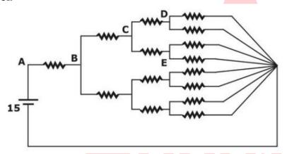
$$R_{DF} = R_{CF} = 2 \parallel 2 = 1\Omega$$
