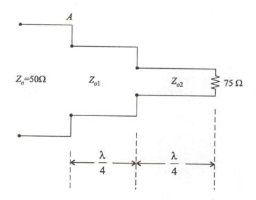
Determine the characteristic impedance  $Z_{o1}$  if  $Z_{o2} = 30 \Omega$  and there is no reflected wave to the left of A.
