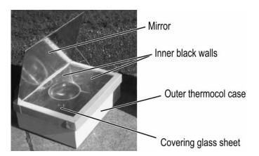
There are three main components to the functioning of most solar cookers:
