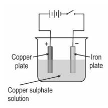
$\frac{Q: 1}{Q: 1}$  After a few minutes, even before he turned the switch on, he noticed that copper was deposited on the iron plate.
