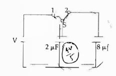
A capacitor of 2  $\mu$ F is charged as shown in the diagram. When the switch S is turned to position 2, the percentage of its stored energy dissipated is:
