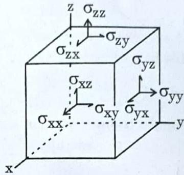
(a) The normal stress components are  $\sigma_{xx}$ ,  $\sigma_{yy}$ , and  $\sigma_{zz}$ . The shear stress components are  $\sigma_{yz}$ ,  $\sigma_{zx}$ ,  $\sigma_{xy}$ ,  $\sigma_{zy}$ ,  $\sigma_{xz}$ , and  $\sigma_{yx}$ . ✓
