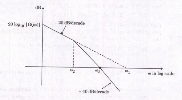
Express the relation between  $\omega_1$ ,  $\omega_2$  and  $\omega_3$ . Also find the static velocity error coefficient  $K_v$  of this system. You can assume  $\omega_2 << \omega_3$ .
