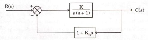
Draw the root-locus with  $K_h = 0$  and K as variable. Obtain the value of K so that the system damping ratio is 0.158.
