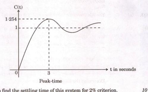
Also find the settling time of this system for 2% criterion.
