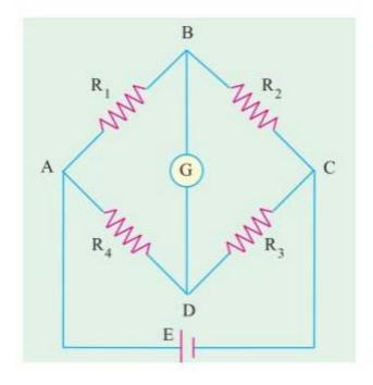
$$\frac{R_1}{R_3} = \frac{R_4}{R_2}$$
