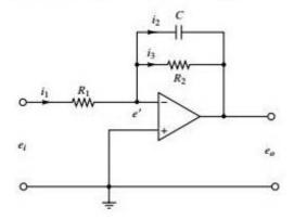
$$\frac{E_o(s)}{E_i(s)} = \frac{R_1}{R_2(R_1Cs + 1)}$$
