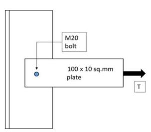
Supposing the drilled holes are used, then the net area for the tension member shown in the figure would be
