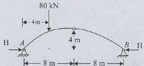
The horizontal thrust of the three-hinged arch loaded as shown in the figure is
