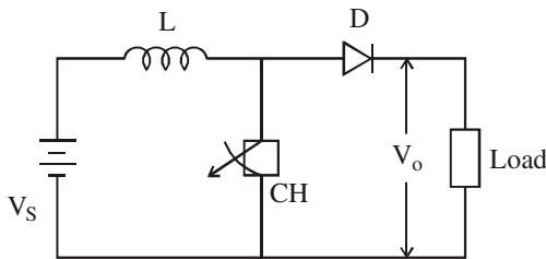
If  $\alpha$  is the duty cycle type and output voltage of the chopper circuit above is
