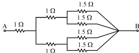
Equivalent resistance between A & B, in the figure above is
