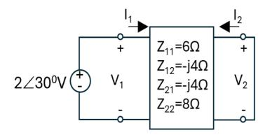
**Ans** X A.  $I_1 = 0.25 \angle (-30^\circ)$  A,  $I_2 = 0.125 \angle 60^\circ$  A
